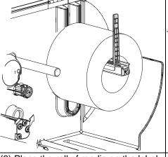
(2) Place the roll of media on the label supply spindle. Flip up the label roll guard. Move the label roll guard horizontally to gently fit the width of
