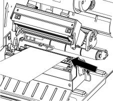
(4)Adjust the label guide to fit the width (5) Unlock the media sensor lock lever of the label.
