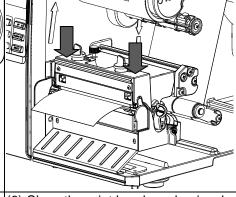
(6) Close the print head mechanism by pushing the both sides of print head mechanism. Make sure the latches are engaged securely.
