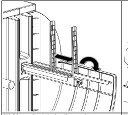
1) Move the label roll guard horizontally to the end of label spindle then flip down the label roll guard.
