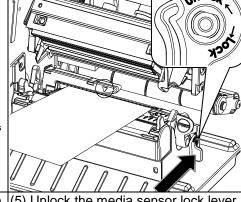
to adjust the media sensor position and lock the media sensor lock lever. (see note below)
